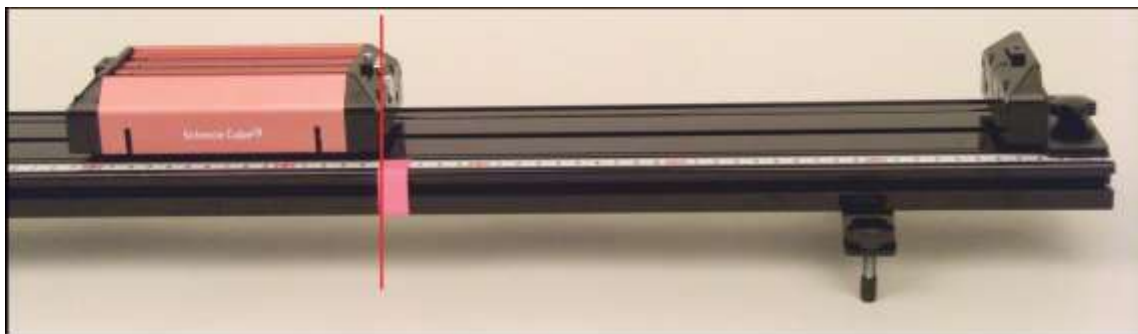
Picture 3.4.15 clicking [Start Experiment] button when the cart is in a certain position: In the process of d and f , start or stop the experiment when the cart enters or goes out the position indicated on the track.
